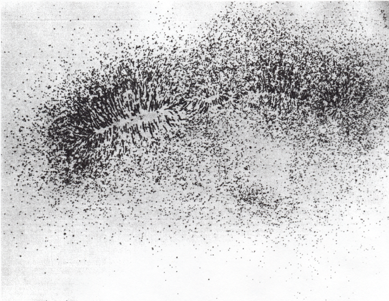
Fig. 2. Photograph of iron filings on white paper against a cut radial tire segment.
